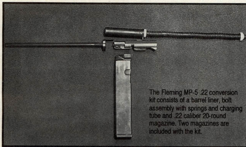
The bolt assembly of the Fleming unit almost mimics the H&K .22 unit with some major improvements. The bolt is equipped with "camming ramps" to eliminate bolt bounce for improved reliability.
